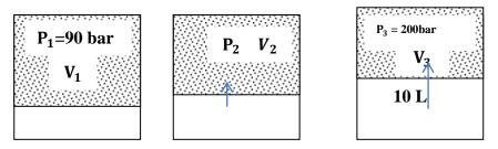
Let precharging pressure be  $P_1$  (90 bar) and  $V_1$ . Gas is compressed by incoming oil from pressure 90 to 200 bar and when the bladder is compressed to 200 bar the volume of oil inside the accumulator is 10 Liters. Therefore we can write.
